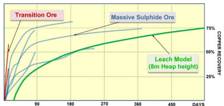
Figure 1. Copper recovery curves from Wetar showing selected column test results and the base case assumption. Source; Finders Resources
