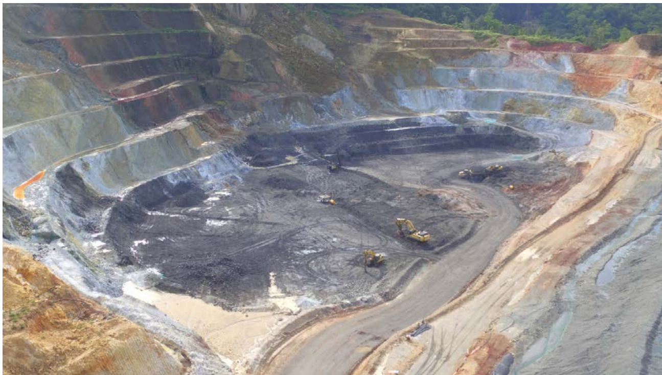
Image 1 – Kali Kuning open pit clearly showing massive sulphides predominating in the pit floor
