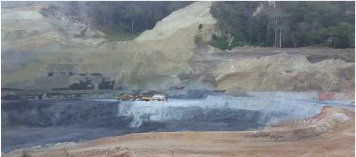
Figure 2: KKV open pit showing the dark high grade ore in contact with light coloured footwall rock.
