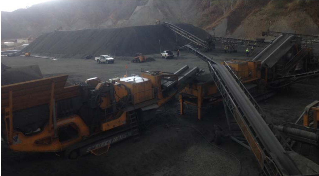
Image 2 – Crusher on KKV leach pad with stacked KKV Heap 1 in the background
